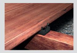
The spacer FTA-IPW/-IPA ensures aquick and invisible installation of decking boards providing a width between 120 – 150 mm. At the same time, an uniform installation pattern is guaranteed. About 15 – 20 pieces are needed per m², depending on board width.
