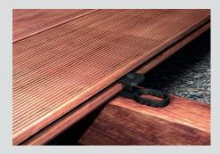
The spacer FTA-ISW/-ISA is suitable for boards with a groove wall thickness of 5.5-11.5 mm and a minimum groove depth of 9 mm. Boards can be installed quick and professionally with an invisible fastening.
