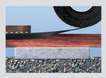
The self-adhesive wood-protection tape FTA-RT is to protect the supporting rail against water. The screw can easily be fixed through the rubber-tape and will effectively seal the fixing point.
