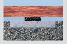
The rubber pats FTA-UP are placed at intervals at certain points under the support rail and will not trap water and dirt.
