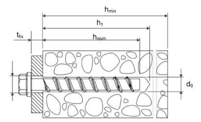
$\begin{array}{lll} d_0 & = & \text{nominal drill bit diameter} \\ h_{\text{nom}} & = & \text{nominal anchorage depth} \\ h_1 & = & \text{depth of the drill hole} \end{array}$
