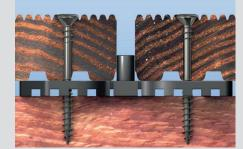
Furthermore, it guarantees spaces between the boards and support rails required for good ventilation. This ensures that any waterlogging that may have occurred can dry out. About 15 – 20 pieces are needed per m<sup>2</sup>, depending on board width.
