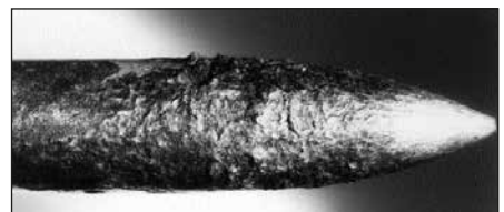
Mechanically cleaned point of a pulled-out DX fastener
