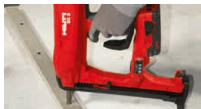
Fastening wood, e.g. Placopan®, to concrete
