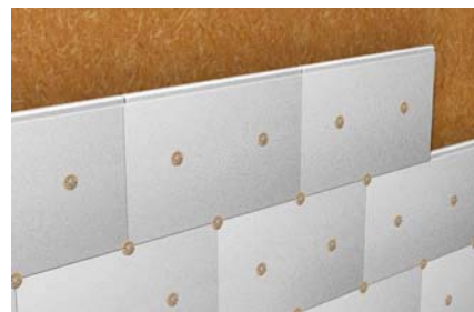
Attachment of polystyrene boards on OSB-panel
